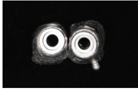
The oxide film can be removed cleanly without damaging the internal side of Hex.
