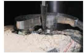
Bar Milling after Casting
