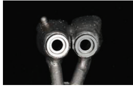
Investment material and the oxide film is removed by using a Glass bead (50um/ 2-4 bar)
